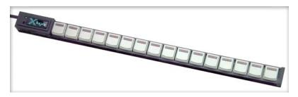
The **X-keys MWII Stick** uses X-keys MacroWorks II software to record key commands from the keyboard and send them to applications on the computer. Any sequence or combination of keystrokes from a standard keyboard may be assigned to any key on the X-keys. Mouse commands (click & scroll) may also be programmed. Simple, intuitive steps allow even non-technical users to program the X-keys instantly. Programming files may easily be copied and shared.
